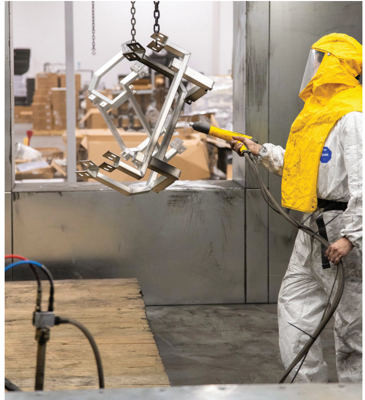
Honor LSV powder coats all of its own frames on-site in a custom built powder coating line that is unique in the industry
