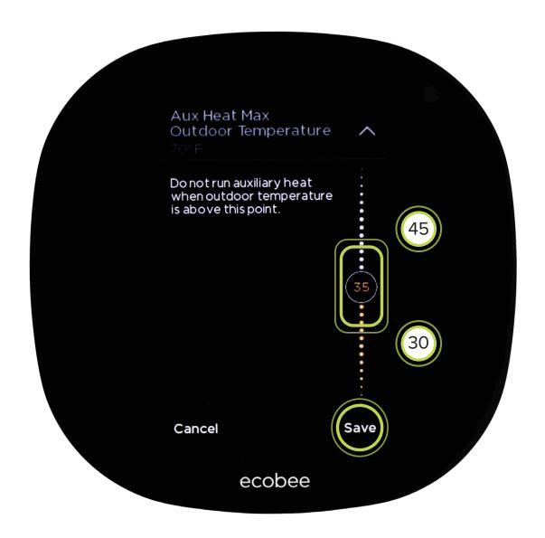
We recommend setting the Aux Heat Outdoor Temperature at 40 degrees to maximize the efficiency of your dual fuel heat pump before gas furnace backup heat comes on to maintain comfort at lower temperatures.
