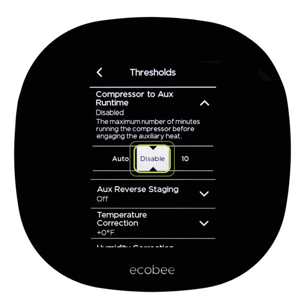
This is to maximize the efficiency of your dual fuel heat pump before gas furnace backup heat comes on to maintain comfort at lower temperatures.
