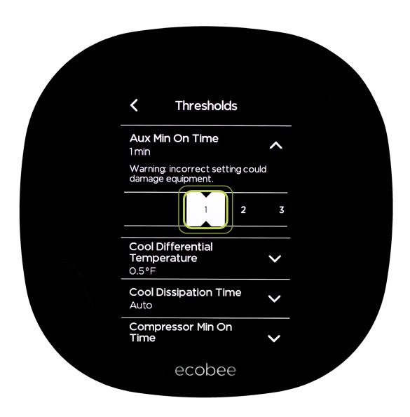
This setting regulates the backup heat runtime, which maximizes energy savings and increases system durability.
