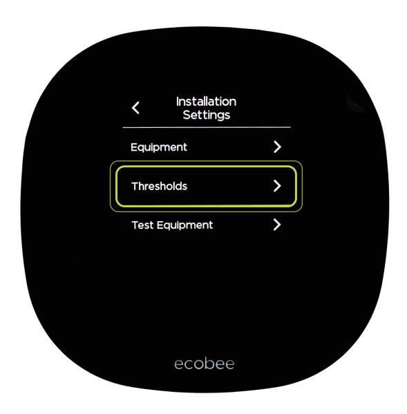
Select Compressor Min Cycle Off Time; select 600 seconds.
