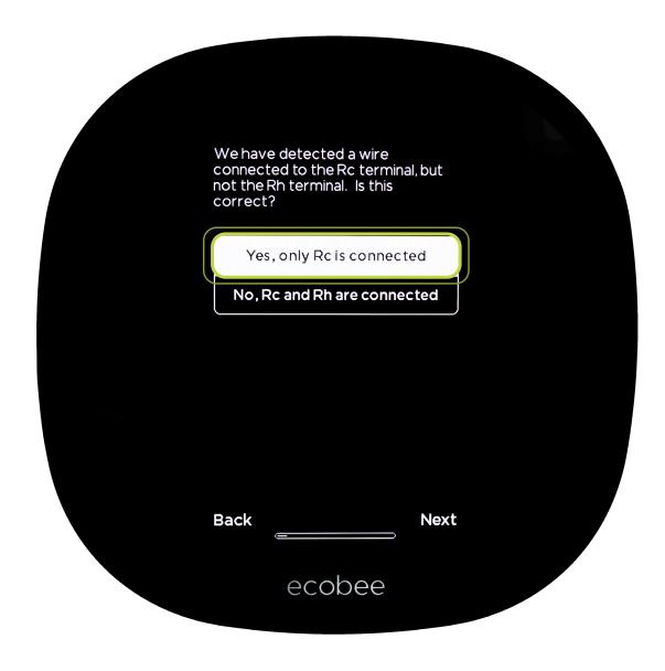
If your HVAC system has two transformers installed, select No, Rc and Rh are connected.
