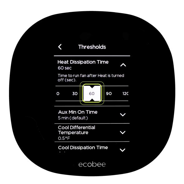
60 seconds will maximize the distribution of remaining heat in the system but not circulate cool air.
