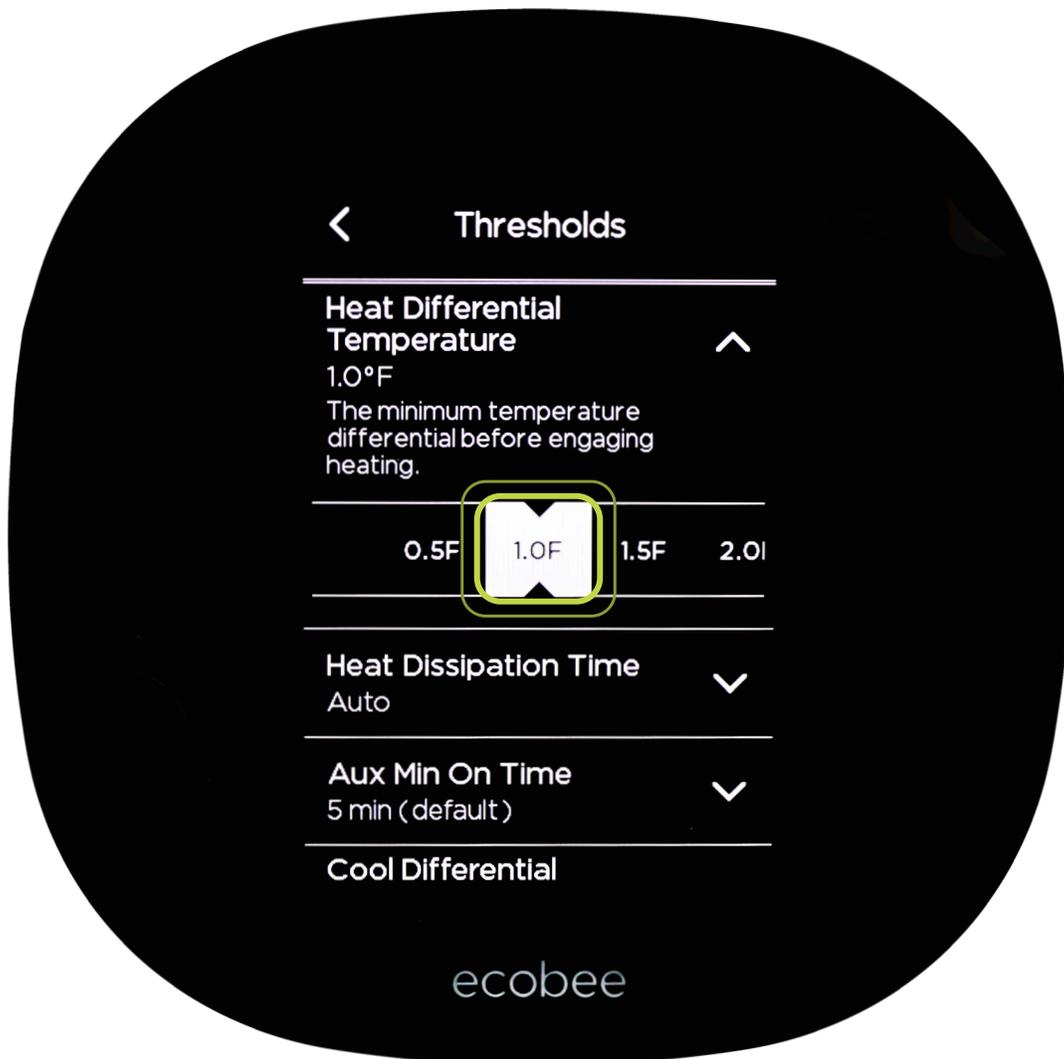
A 1°F heat differential temperature will turn the heat on after the indoor temperature drops 1°F below setpoint. This setting should decrease energy usage and increase system durability through longer runtimes.
