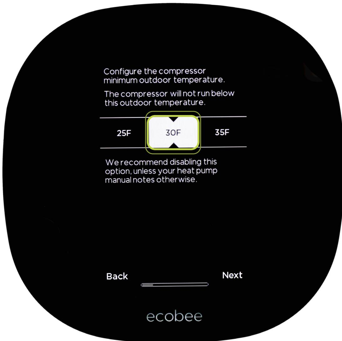
We recommend setting the minimum compressor at 30 degrees to maximize efficiency. This is the outdoor temperature at which your dual fuel heat pump switches over to your gas furnace backup heat to maintain comfort at lower temperatures.
