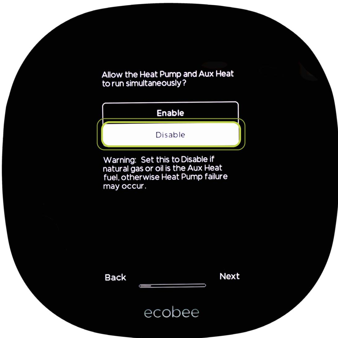
This is the recommended setting to keep your heat pump from running at the same time as your gas furnace backup heat to maintain comfort at lower temperatures.
