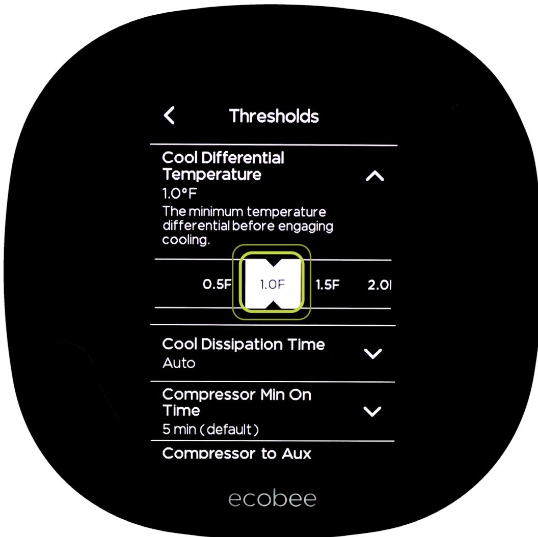
A 1°F cool differential temperature will turn the cooling on after the indoor temperature is 1°F above setpoint. This setting should decrease energy usage and increase system durability through longer runtimes.
